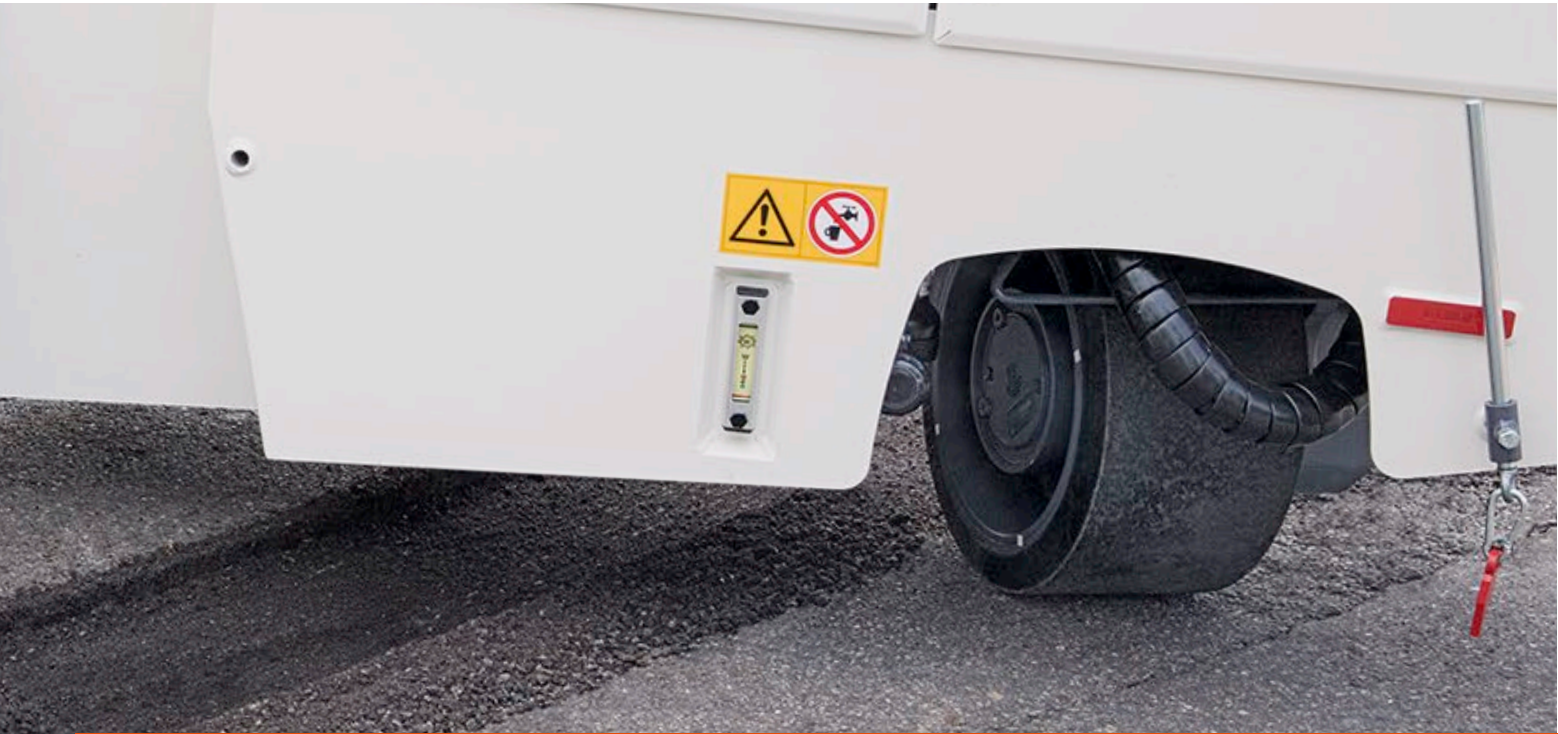
01 - 02 The electronically controlled travel drive makes high-precision milling possible - such as around road installations, for example.
