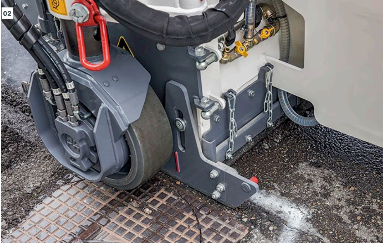
01 - 02 The electronically controlled travel drive makes high-precision milling possible - such as around road installations, for example.
