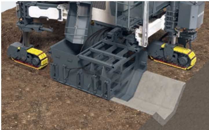
Embedded V-profile drainage channel, paving left
