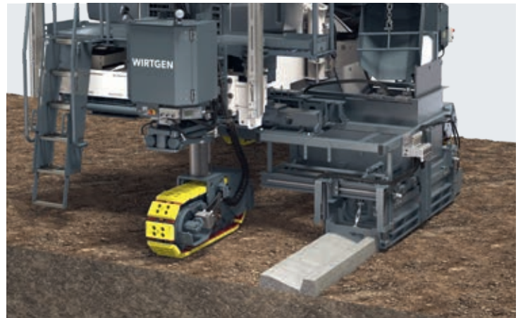
Special profile with combined paving mold, paving right
