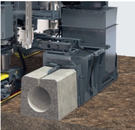
Slot drain, paving right
