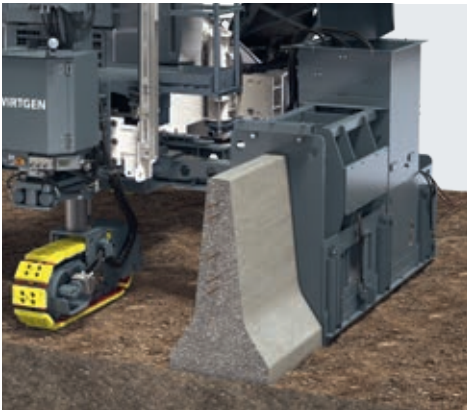
Concrete safety barrier, paving right
