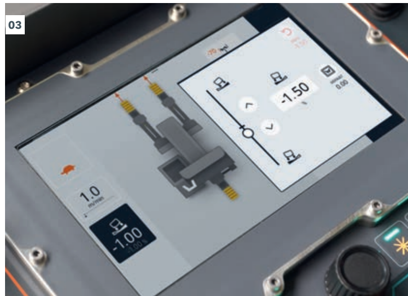
03 ... or the cross slope can be conveniently set from the main control panel.
