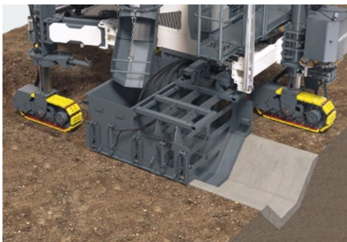
Embedded V-profile drainage channel, paving left
