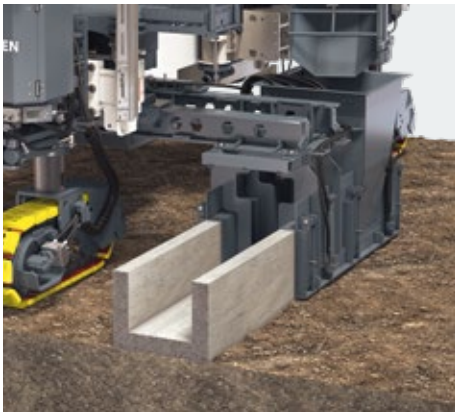
Free-standing U-profile channel, paving right
