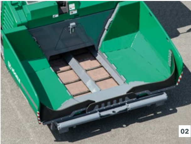
01 Independently operated hopper wings. 02 The large material hopper holds 14.3 tons (13 tonnes).
