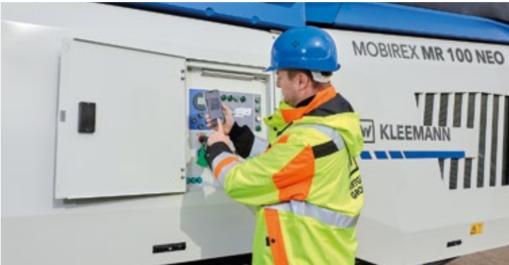
1. Connect the MR 100 NEO with SPECTIVE CONNECT by simply scanning the access data from the machine's display.
