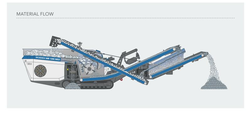
The MR 100i NEO/NEOe stands out with its very high final product quality. This is guaranteed not only by the powerful crushing unit with its 4-ledged rotor with a large impact range and versatile rotor ledge variants, but also by the 5" x 10' 2" large, single-deck post screening unit. This enables the production of a classified final grain size. Thanks to integrated oversize grain returning,
