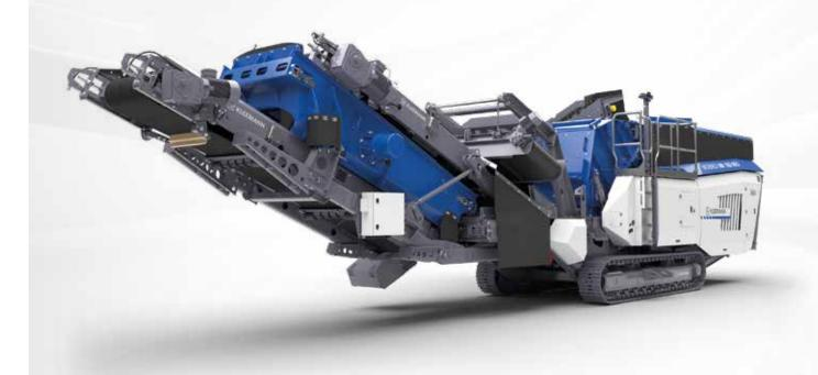
**Track-mounted impact crusher**For use in recycling and natural stone
