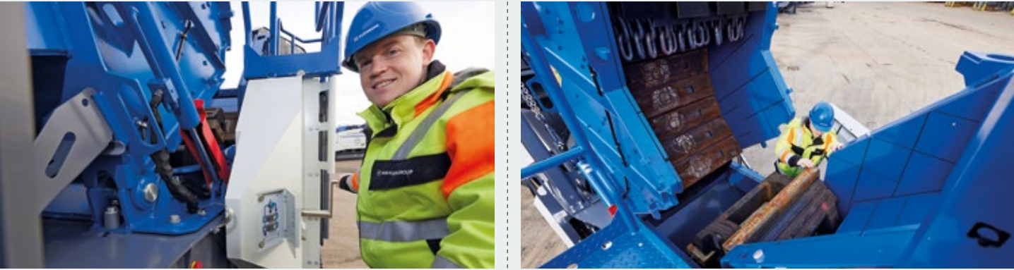
> The rotor is moved into position for wear check or rotor ledge replacement. The crusher is opened completely for best possible access for service and maintenance from both sides. Rotor ledge replacement takes place easily from above.
