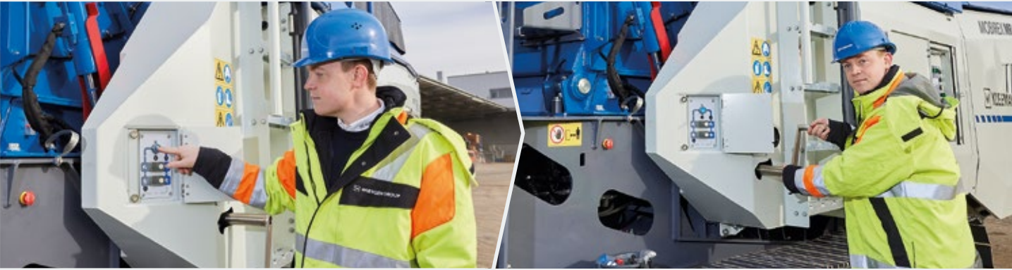
> The rotor locking and turning device is released at the touch of a button... ...and engaged by hand crank.
