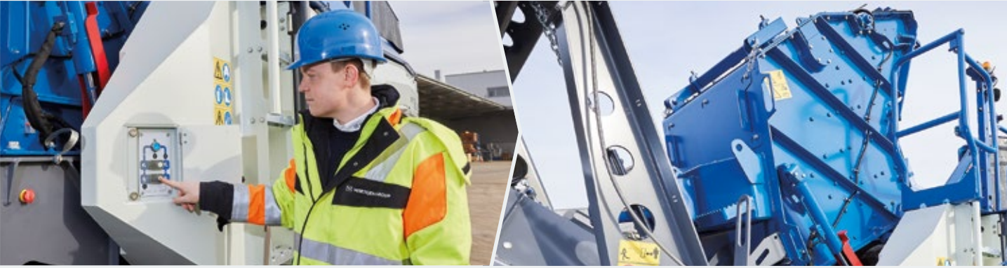
> Automatic opening of the crusher housing when the button is held down... ...until the crusher opens completely. The mechanical safety catch also engages.
