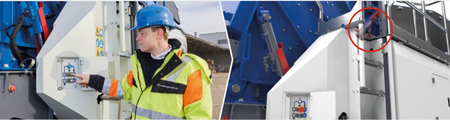
> The crusher is unlocked at the push of a button... ...and the wedges for locking the crusher housing are pulled hydraulically.
