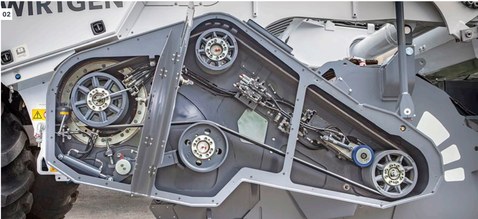
02 Belt drive for the crushing and mixing rotor.
