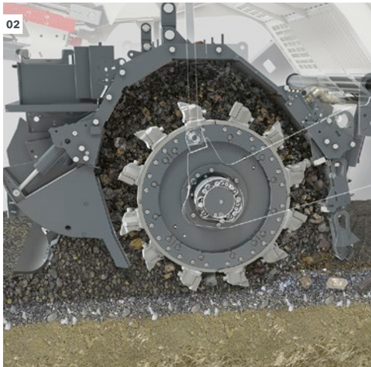
02 - 03 To guarantee optimal mixing results, the WRC 240(i) features a variable mixing chamber like that of the WR Series models.
