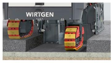
Milling drum assembly FB1500 with Multiple Cutting System MCS BASIC.
