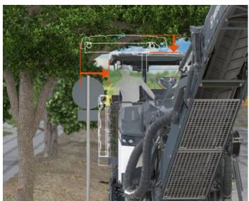
The vertically and horizontally adjustable weather canopy provides optimum protection in a range of different working positions - especially on construction sites with restricted space.
