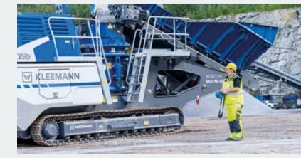
The MOBICONE MCO 90i EVO2 mobile cone crusher has a high constant crusher drive power of up to 248 hp and a maximum of up to 355 hp. This enables a continuous crushing process and higher production volume in special applications. Thanks to a short heating-up phase of the lube oil, the plant is quickly ready
