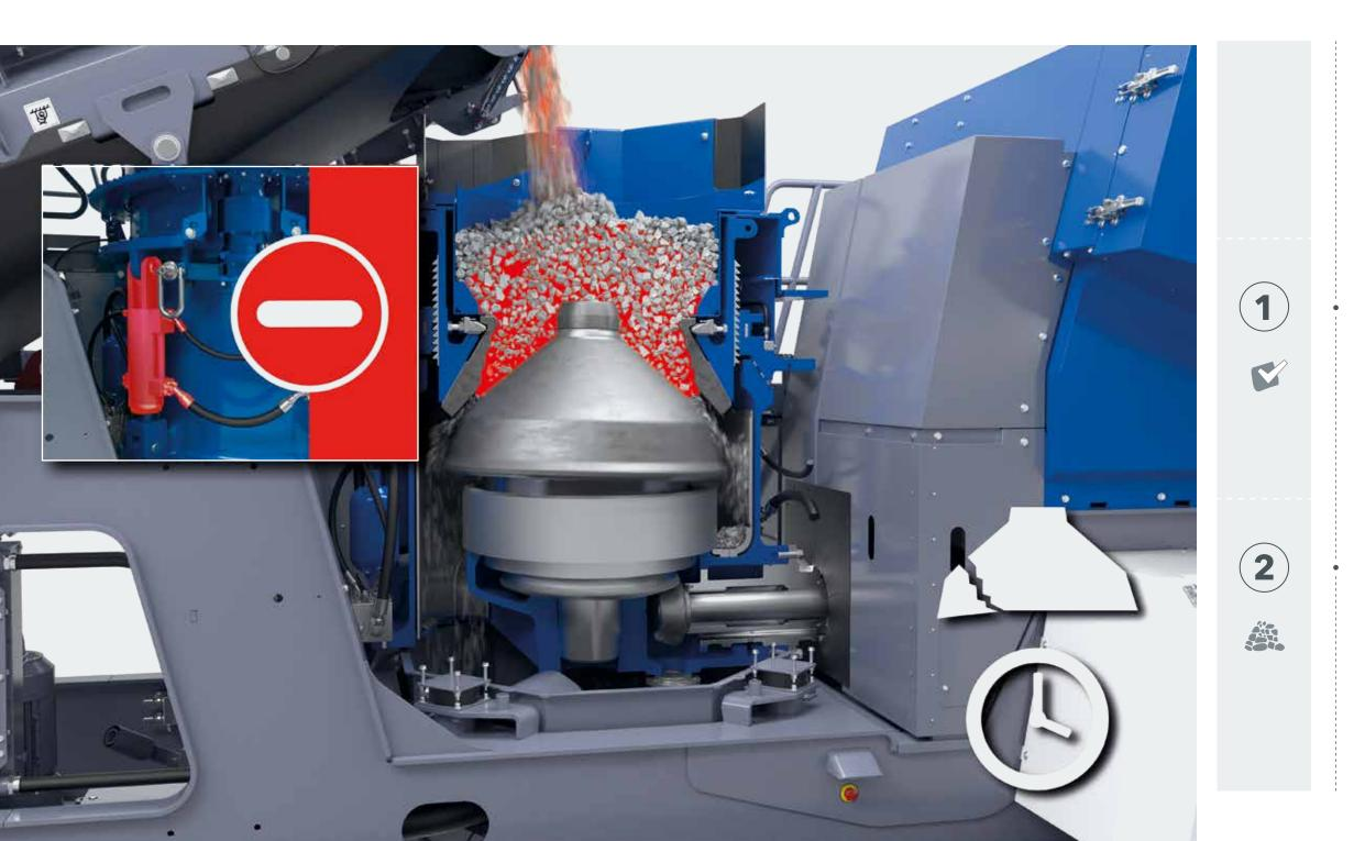
The bowl including the bowl liner lifts to allow uncrushable material to fall through - and the plant remains protected.
