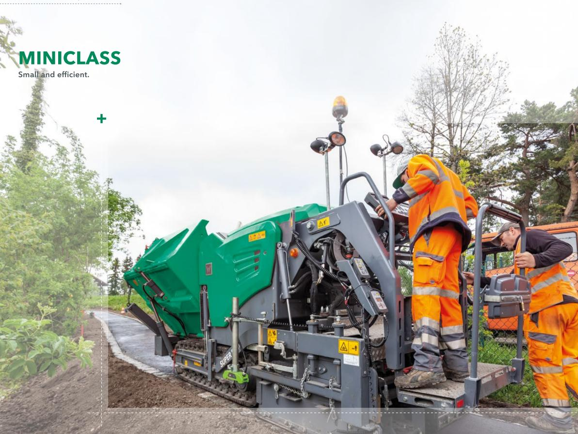
up to 10 ft 6 in (3.2 m) Pave width up to 275 tons/h (250 tonnes/h) Laydown rate
