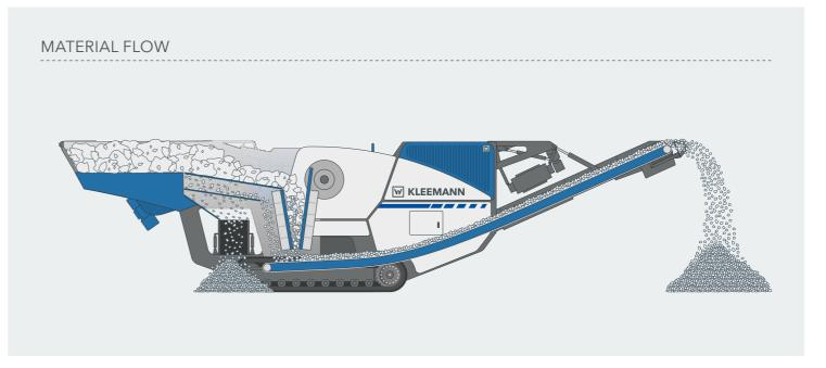
With its low weight and very compact dimensions, the MOBICAT MC 100(i) EVO can be used directly on site - even at narrow or hard-to-reach construction sites in urban areas. Short set-up times are also ensured thanks to feeding unit integrated in the chassis, which means that
