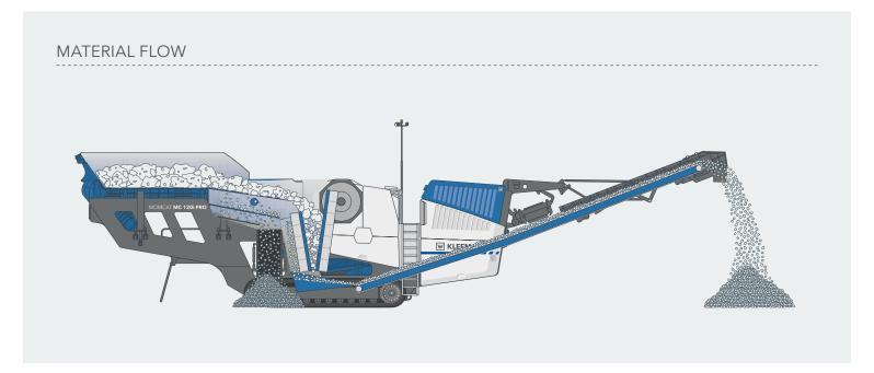
The MOBICAT MC 120i PRO has a generously dimensioned feeding unit, which enables large quantities of materials to be fed using an excavator or wheel loader without any difficulty. The plant's high level of performance is also reflected by the dimensions of the crusher inlet and the extra-long moving crusher jaw design.
