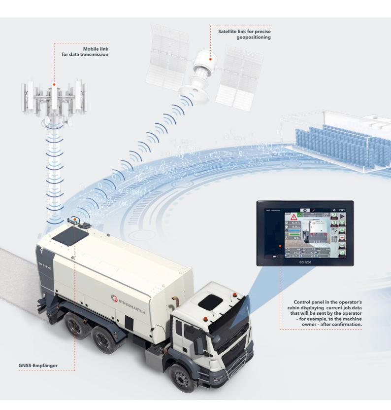
**01** The operator receives constant information about the current machine and job parameters and, at the end of the working day, this data is transmitted to the machine owner simply by pressing a button.
