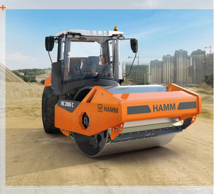
The HC series compactors are powerful professionals with a big compaction force. The 3-point articulation and large slope angle front and back make them extremely maneuverable whilst ensuring optimum driving stability. The HC series is well prepared for the quality and communication requirements of the future with interfaces and hardware.
