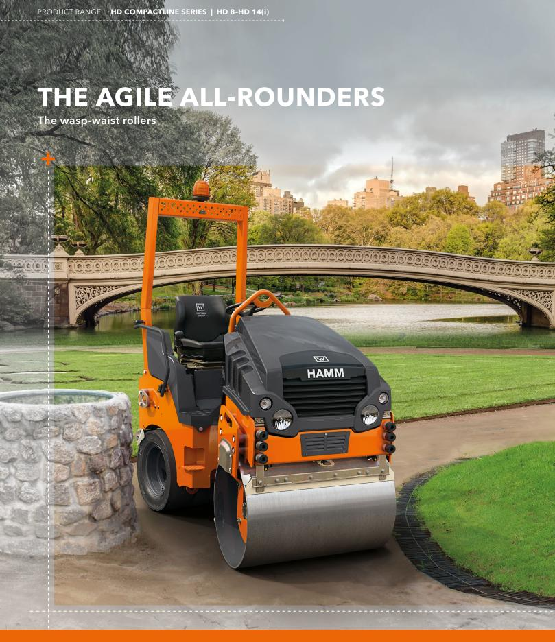
The articulated compact rollers in the HD CompactLine series are all-rounders for asphalt construction, earthworks and landscape gardening. Their operation is extremely easy and calls for no special language skills. The wasp-waist design provides optimal visibility, and the 3-point articulation ensures outstanding driving and handling characteristics.
