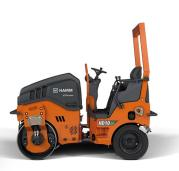
In terms of operation and compaction power, the eight fully electrically driven tandem rollers from HAMM are identical to their sister models with combustion engines. Thanks to the electric drive, they work on construction sites with zero local emissions and with significantly reduced noise.
