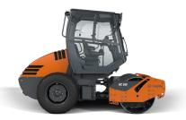
The extremely compact, very short compactors of the HC CompactLine series offer a huge gradeability of up to 60% and maximum ground clearance. They are driven by modern wheel motors. The very short wheelbase and 3-point articulation ensure optimal driving and handling characteristics - ideal for cramped construction sites and for compaction on rough terrain.
