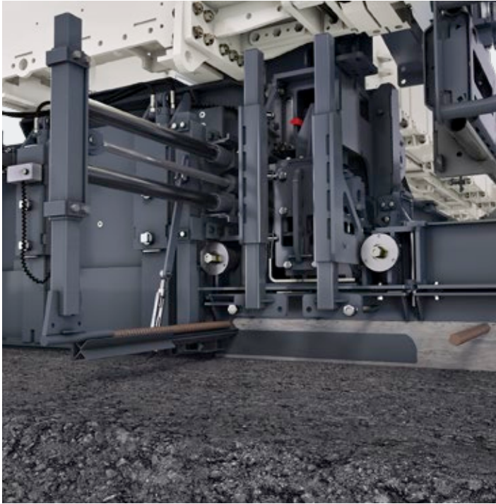
Separate side tie-bar inserter.
