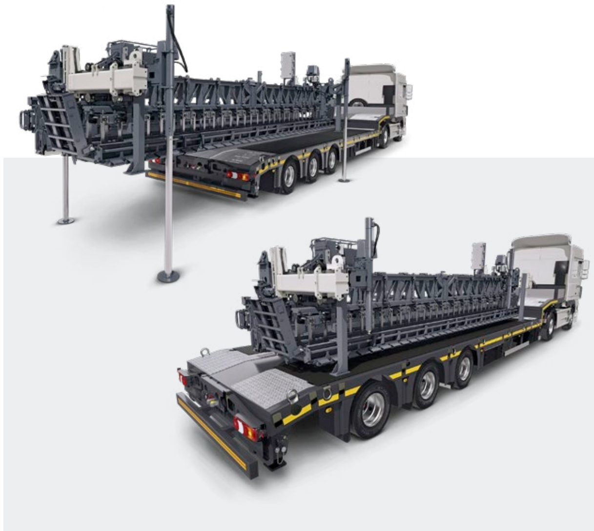
Self-loading dowel bar inserter.
