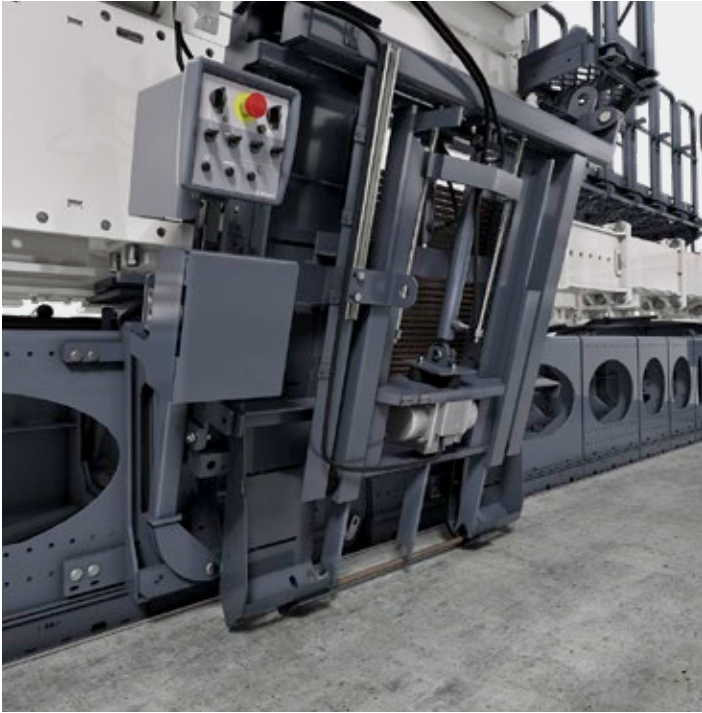
Longitudinal tie-bar inserter with control unit.
