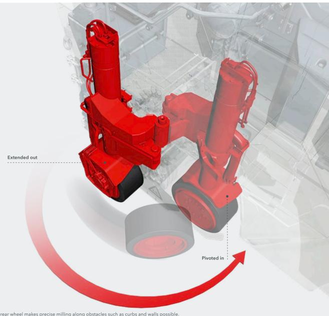
When pivoted in, the right rear wheel makes precise milling along obstacles such as curbs and walls possible.
