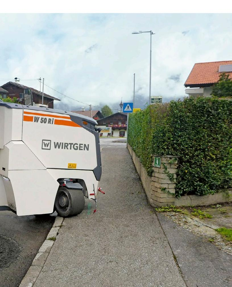
The most powerful half-meter cold milling machine features an efficient operating concept at a working width of 20 in (0.5 m) or 2 ft (0.6 m). Easy-to-use additional and automatic functions increase the machine's performance potential to quickly complete any milling job. The machine can be equipped with a large number of different milling drums, in-creasing flexibility and machine utilization.
