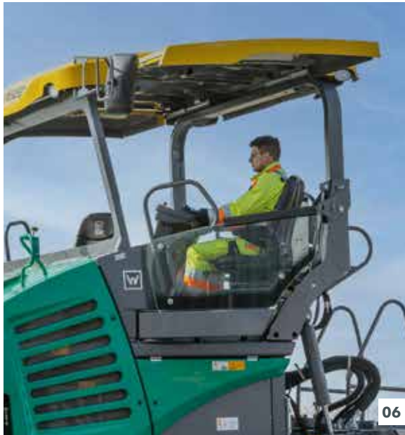
04 Safe and convenient step. 05 VÖGELE EcoPlus low-emissions package significantly reduces fuel consumption and noise levels. 06 The paver operator's platform ensures maximum visibility.
