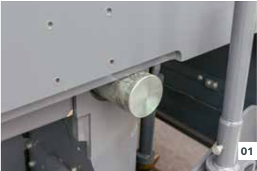
01 Locking bolts on both sides secure the screed in its transport position. 02 When the screed is in the floating position, the Screed Assist feature can also be activated. 03 Screed plates are fitted as standard with heating elements which distribute the heat all over the plates.
