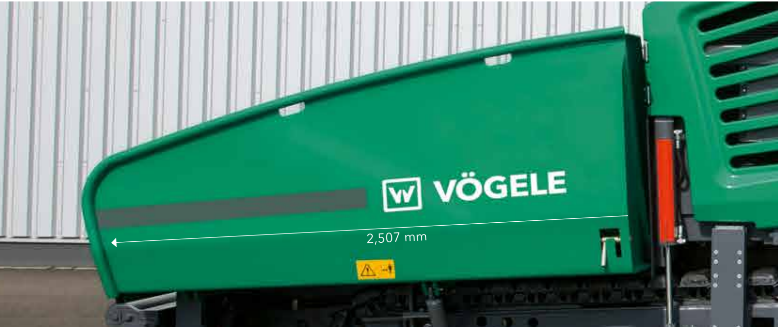
Large material hopper holding 15 tonnes specially adapted to the feed vehicles used as standard in China
