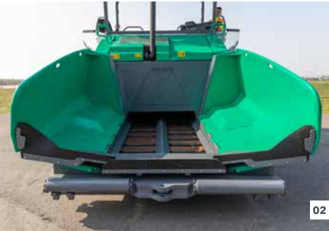
01 Choice of engine speed ranges 02 The two hopper sides can be folded separately or both together at the push of a button.
