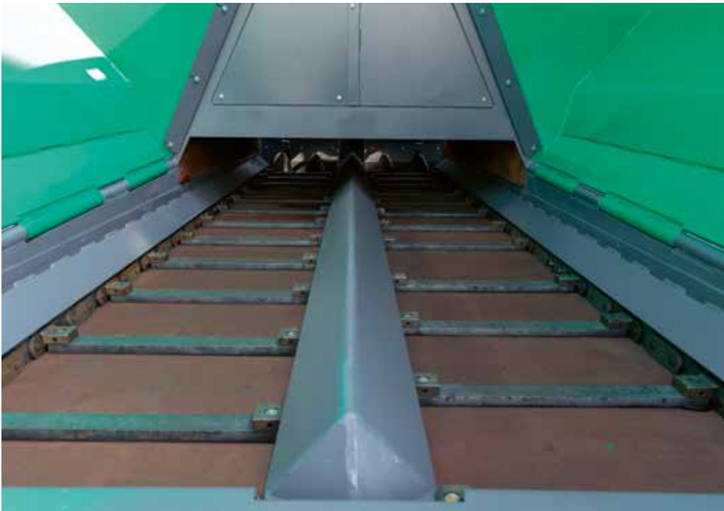
The conveyor can be reversed at the push of a button. The return transport of the mix is automatically stopped. The conveyor can be switched to the no-load function just as quickly.
