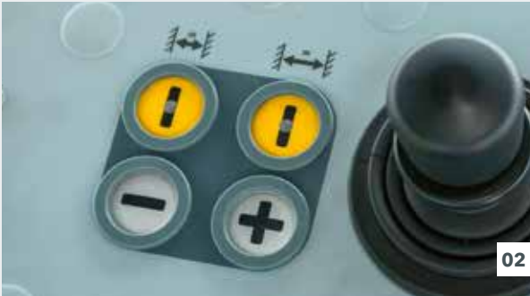
For automatic distance control the operator can select between two different distances.
