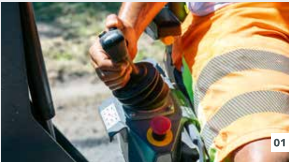
The pivoting conveyor is controlled via a joystick in the armrest of the operator's seat.
