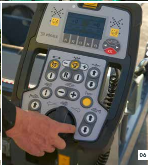
04 PaveDock Assistant communication system for optimum material feed 05 Large material hopper with a capacity of 13 tonnes 06 ErgoPlus 3 screed operator's console with SmartWheel for convenient screed width control
