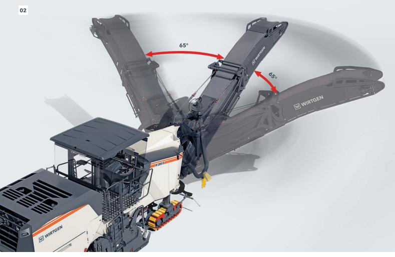
**01** Increased scraper lift for a wider range of milling applications and reduced wear. **02** Large slewing range of the discharge conveyor.
