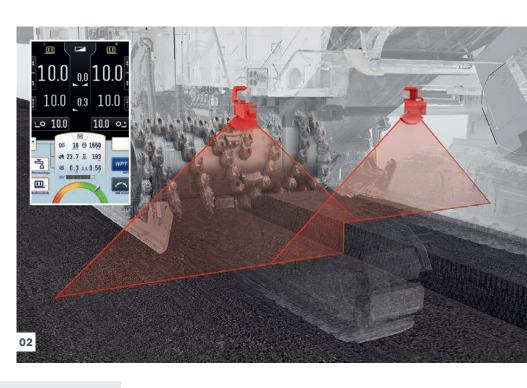
The current milling volume and truck tonnage are continuously displayed to the machine operator on the 7" control panel during the milling process.
