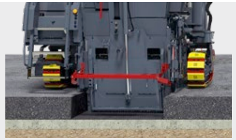
W 130 Fi with 1.3-m milling drum unit
