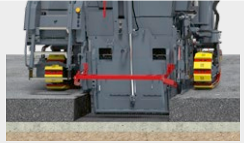
W 130 Fi with 1.3-m milling drum unit
