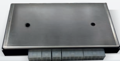
Computer unit in the central electrical system
