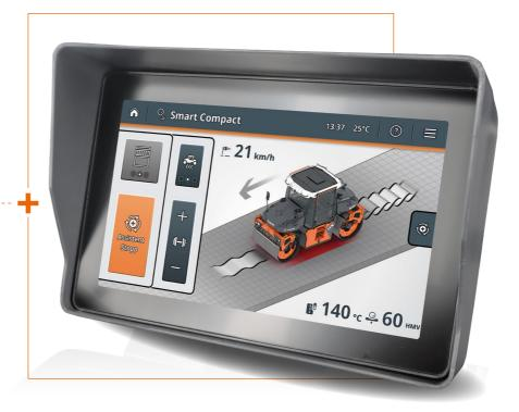
Data is input and output via the additional Smart Display on the dashboard. This is where the driver sees the layer that is currently processed, the direction of travel, the wind speed, the asphalt temperature, the compaction value (HMV), and the current compaction settings for each drum.
