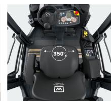
On request, the driver's seat can be electrically operated, allowing it to be moved and swivelled by up to 350°.
