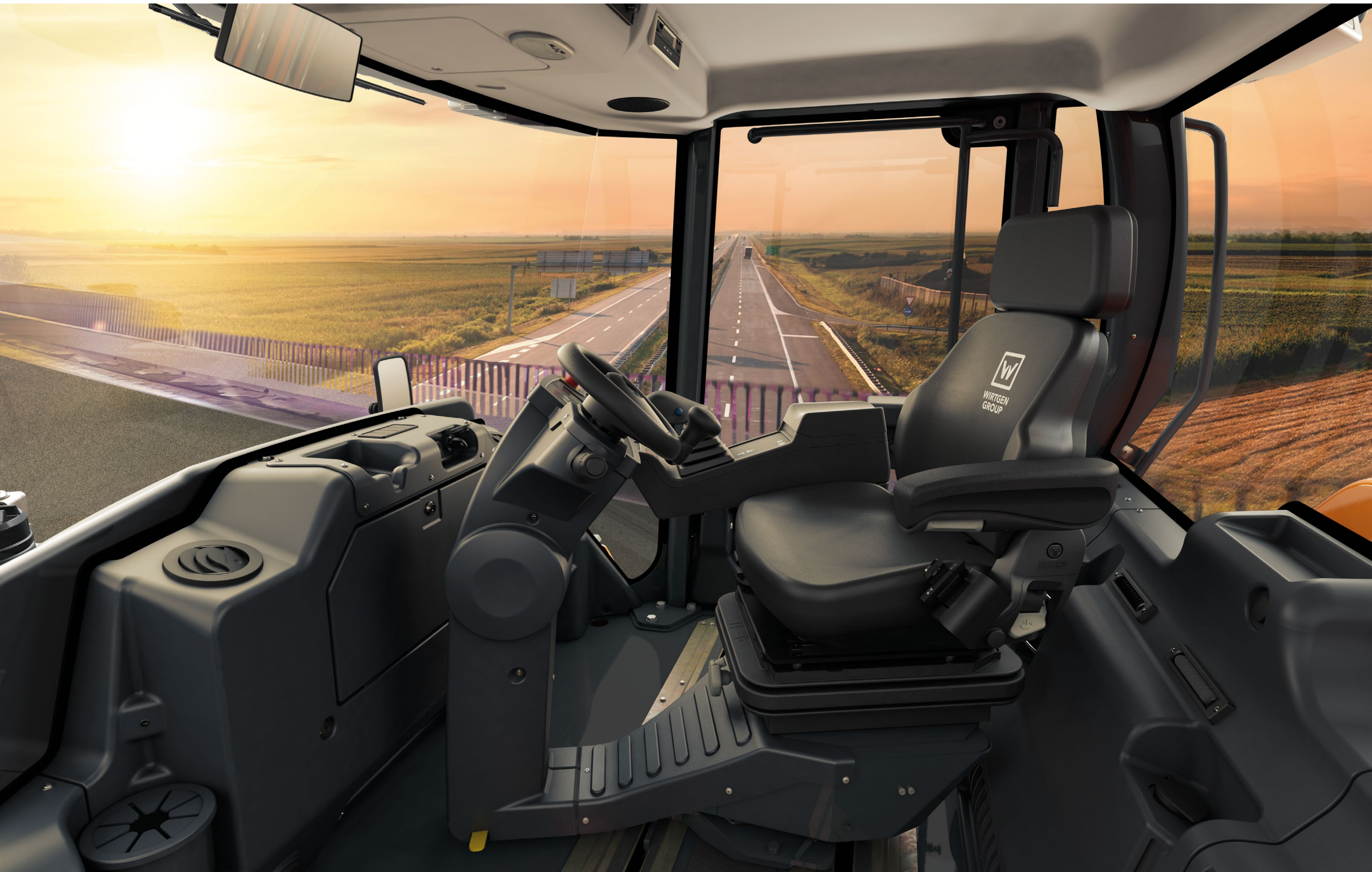
The tilt of the dashboard and steering wheel can be individually adjusted.
