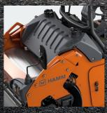
The open frame and the shape of the tanks provide an unobstructed view of the area directly in front of the drums.
