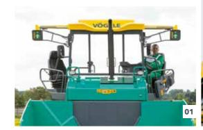
01 The paver has two sets of signal lights, mounted on the left and right of the hardtop. 02 The paver operator can indicate clearly whether the truck driver is to reverse, stop or dump mix, for example. 03 The signal is conveniently selected straight
