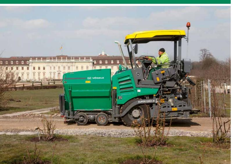
The separate hydraulic drives in both rear wheels and two front wheels ensure maximum power transmission. Electronic Traction Management and an electronically limited slip differential acting on the drives of the rear wheels assure optimum traction, even on difficult terrain.
