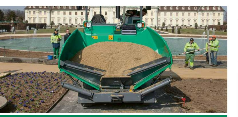
Large material hopper with a capacity of 10 tonnes
