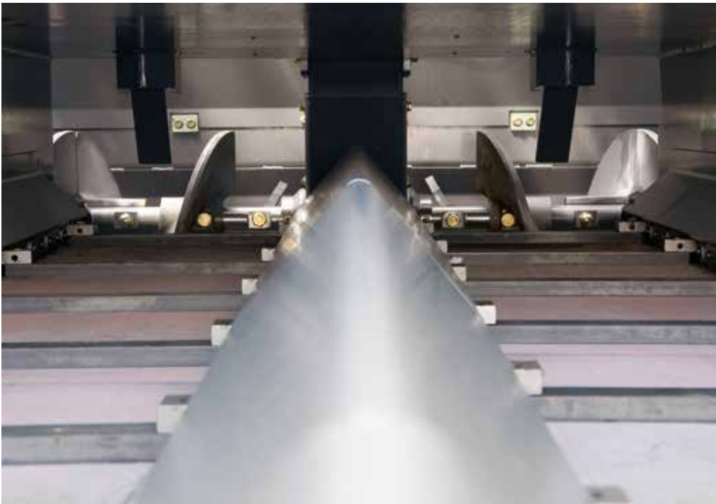
The conveyor can be reversed at the touch of a button. Return transport of the mix is stopped automatically. The conveyor can be switched to the no-load function just as quickly.
