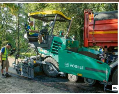
01 ErgoPlus 3 operating system with numerous convenient and automatic functions. **02** Wheeled paver with a large range of applications.
