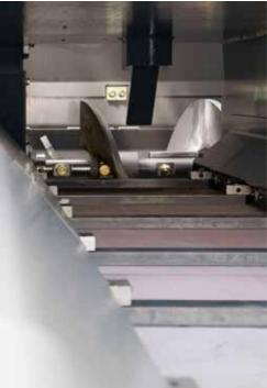
The conveyor can be reversed at the touch of a button. Return transport of the mix is stopped automatically. The conveyor can be switched to the no-load function just as quickly.
