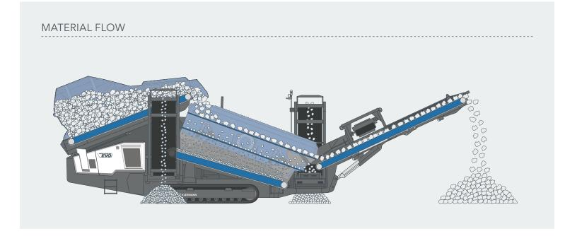
With its proportionally controlled chassis, the coarse screening plant can be moved quickly and precisely, to the application site or within the construction site. The side discharge belts can be folded without the need to assemble or disassemble any components, thereby reducing set-up times. More versatility is achieved thanks
