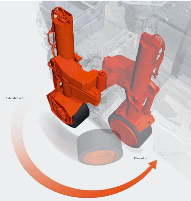
When pivoted in, the right rear wheel makes precise milling along obstacles such as curbs and walls possible.
