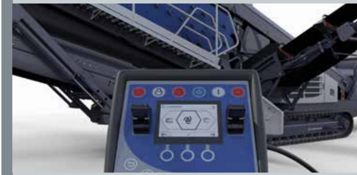
Mobile control panel
