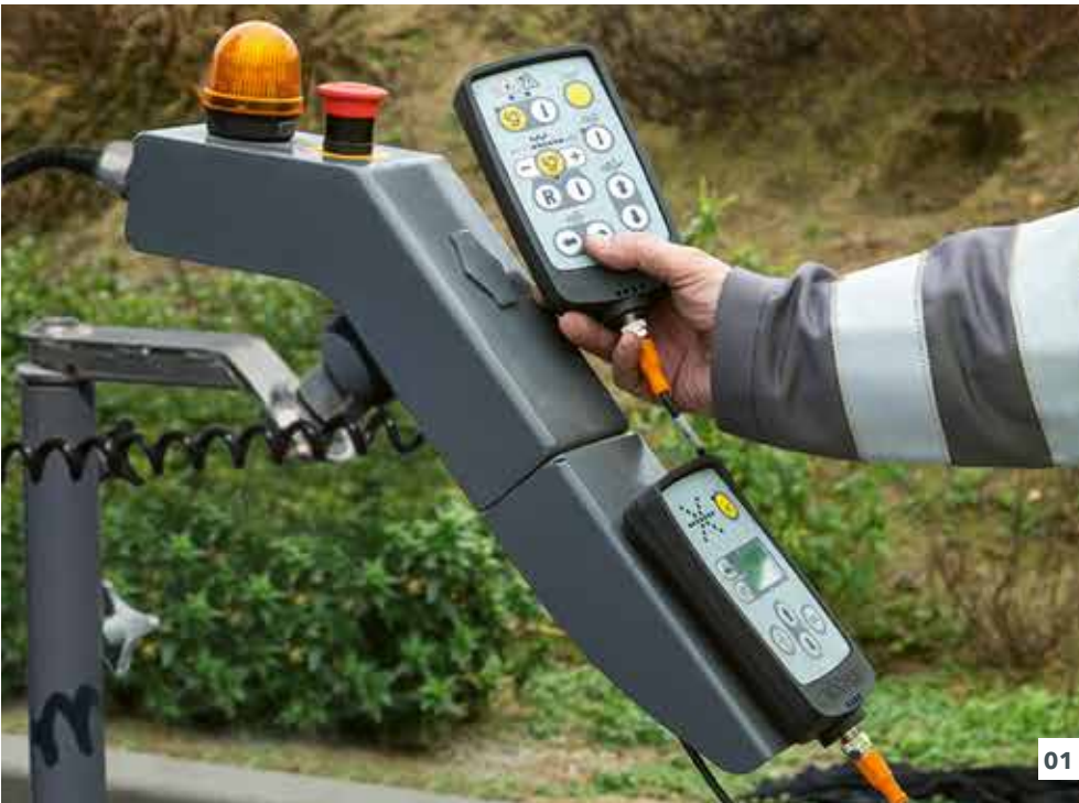
01 Screed width control The screed width on one side can be adjusted at the touch of a button at any time.
