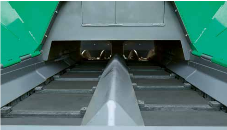
01 Proportional control and continuous monitoring of augers guarantee a constant head of mix in front of the screed in line with current requirements.
