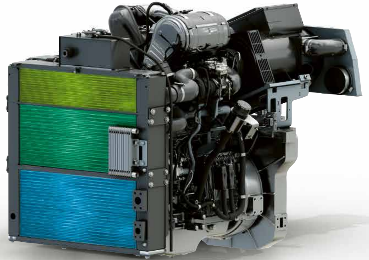
■ = Hydraulic oil ■ = Coolant ■ = Charge air
