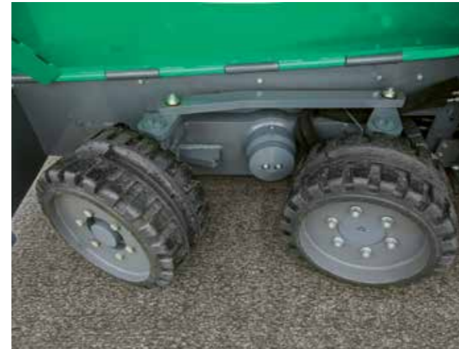
Front wheels mounted on bogies. They provide for a continuous ground contact of the wheels also when working on an uneven base.
