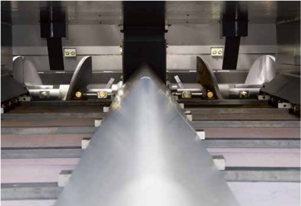
The conveyor can be reversed with just one button push. The mix return stops automatically. The conveyor can be set to idle mode just as quickly.
