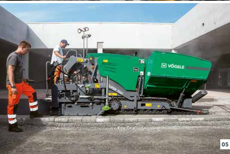
01 Large material hopper with 12,790 lbs. (5.8 metric tonnes) capacity. 02 Positive tracking and precise steering thanks to closed-loop traction drive. 03 Easy handling with the innovative user-friendly ErgoBasic operating concept. 04 All key paving functions can be controlled on the two handy screed remote control units.
