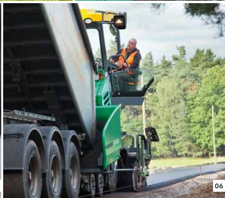
04 The paver operator's platform ensures maximum visibility. 05 Automated processes with AutoSet Plus. 06 Optimum feeding with mix thanks to the large material hopper and PaveDock Assistant communication system.
