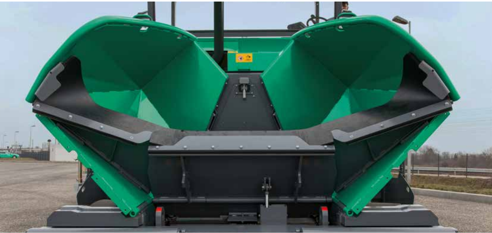
Large material hopper with a capacity of 13 tonnes
