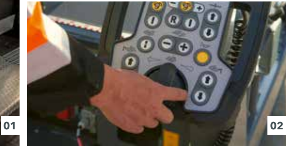
01 The high-contrast colour display provides for brilliant readability even in poor lighting conditions. What's more, the downward-angled high-power LED lighting gives the operator a perfect view of all processes associated with the side plate, even in the dark. 02 Screed width can be adjusted by means of the SmartWheel.
