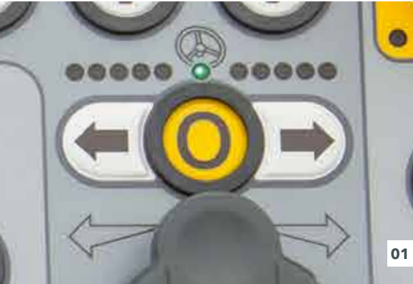
01 For long curves with a constant radius, the desired steering angle can be preselected using arrow keys.
