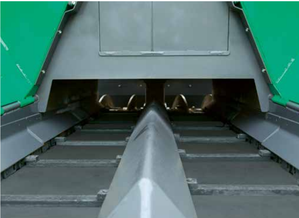
The conveyor can be reversed at the touch of a button. Return transport of the mix is automatically stopped. The conveyor can be switched to the no-load function just as quickly.
