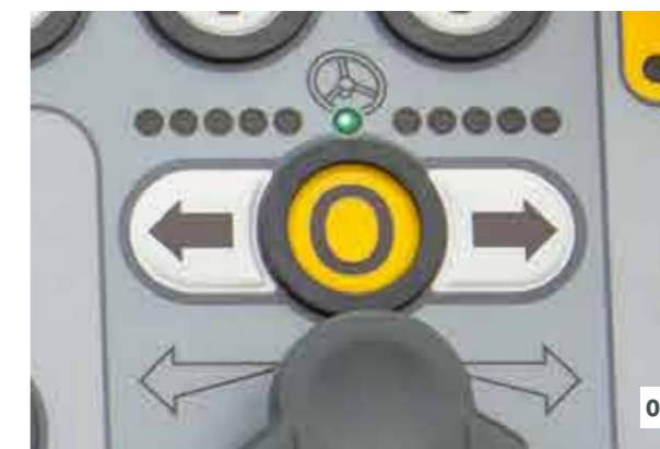
01 For long curves with a constant radius, the desired steering angle can be preselected using arrow keys.
