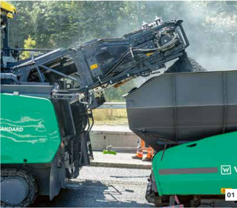
01 Mechanical distance control is also available for the MT 3000-3(i) Standard as an alternative to laser-controlled distance control. 02 Laser-controlled distance control for VÖGELE PowerFeeders consists of three individual laser sensors.
