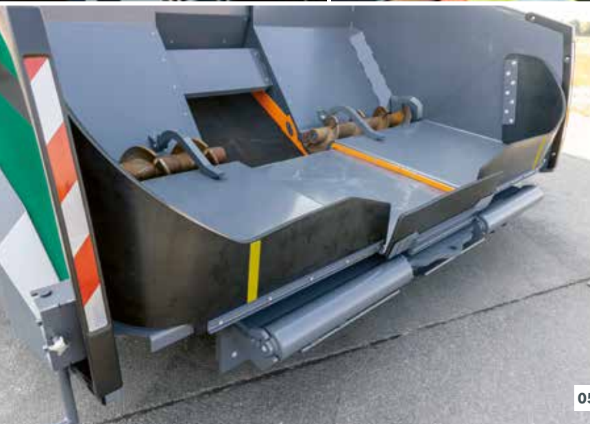
01 Classic material feeding with the MT 3000-3(i) Standard 02 Non-contact transfer of mix 03 PaveDock Assistant truck communication system 04 Operator's ErgoPlus 3 console 05 Redesigned material hopper 06 New service and maintenance concept
