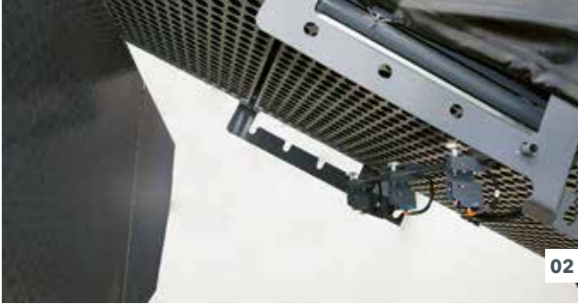
01 Mechanical distance control is also available for the MT 3000-3(i) Standard as an alternative to laser-controlled distance control. 02 Laser-controlled distance control for VÖGELE PowerFeeders consists of three individual laser sensors.
