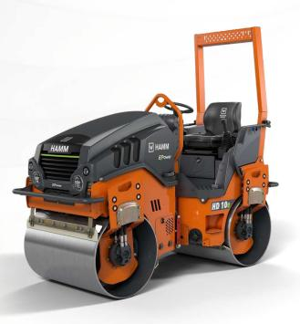
Tandem rollers Series HD CompactLine Tandem roller with two vibrating roller drums H289
