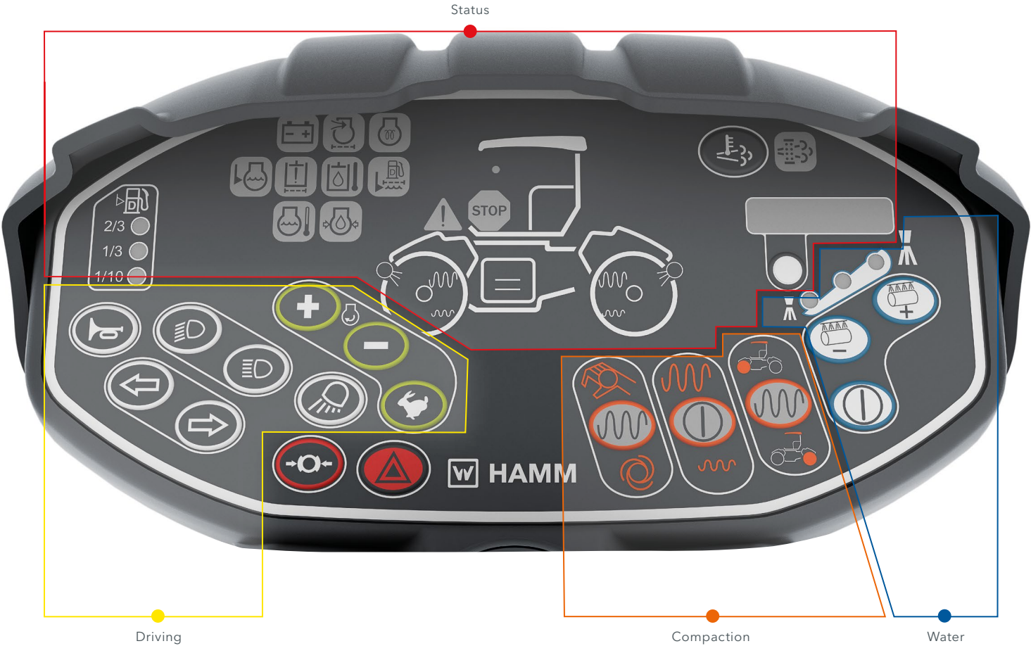
The operator's display, designed with clear symbols, ensures easy operation - without the need for any language skills. The display clearly shows the machine's status and indicates fault signals.
