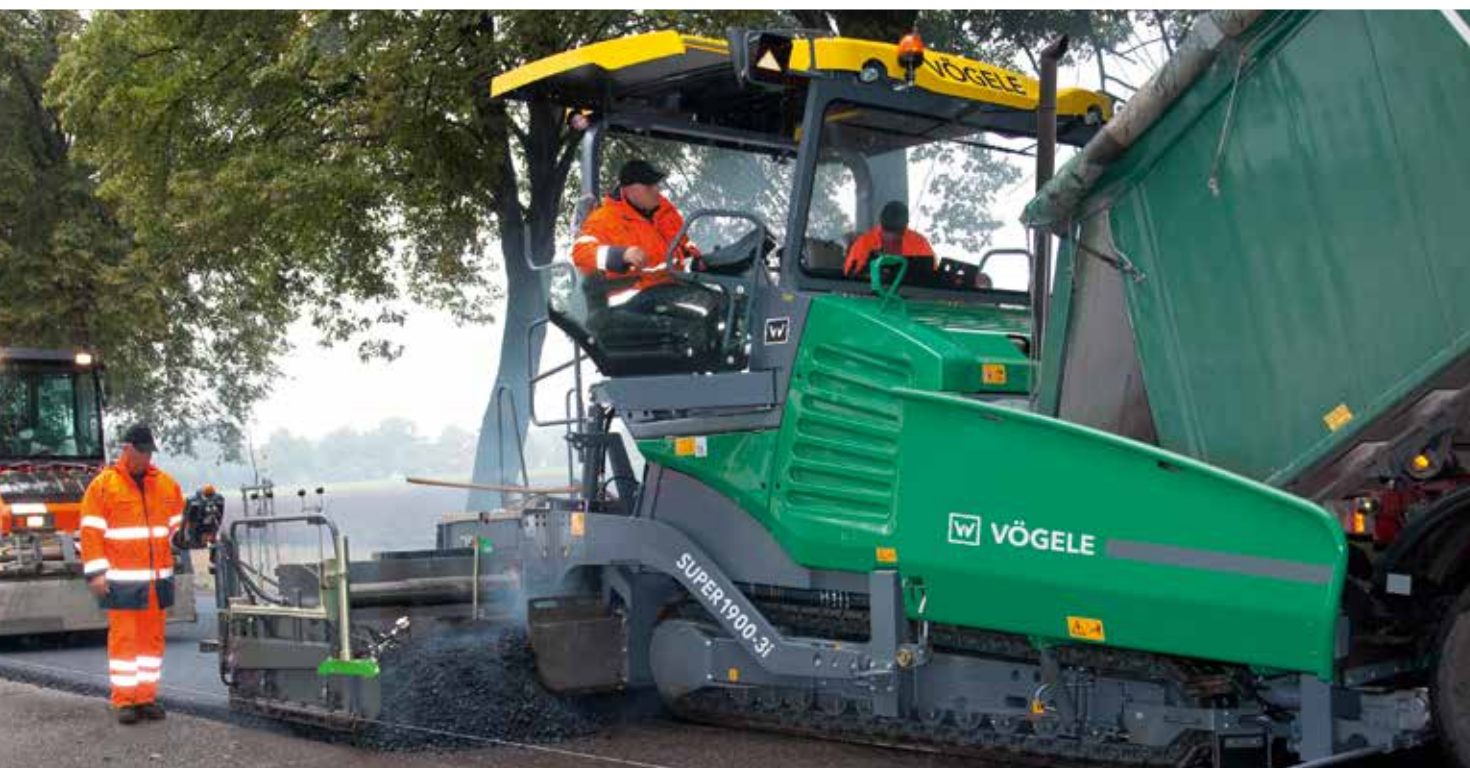
The power unit of the SUPER 1900-3i with its diesel particulate filter (DPF), diesel oxidation catalyst (DOC) and selective catalytic reduction (SCR) for exhaust gas after-treatment complies with the strict requirements of European exhaust emissions standard Stage V and US EPA standard Tier 4f.
