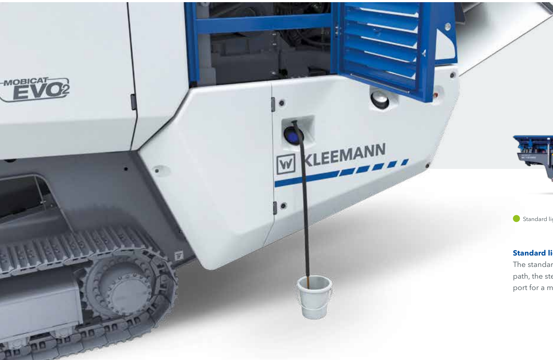
Central drain point
