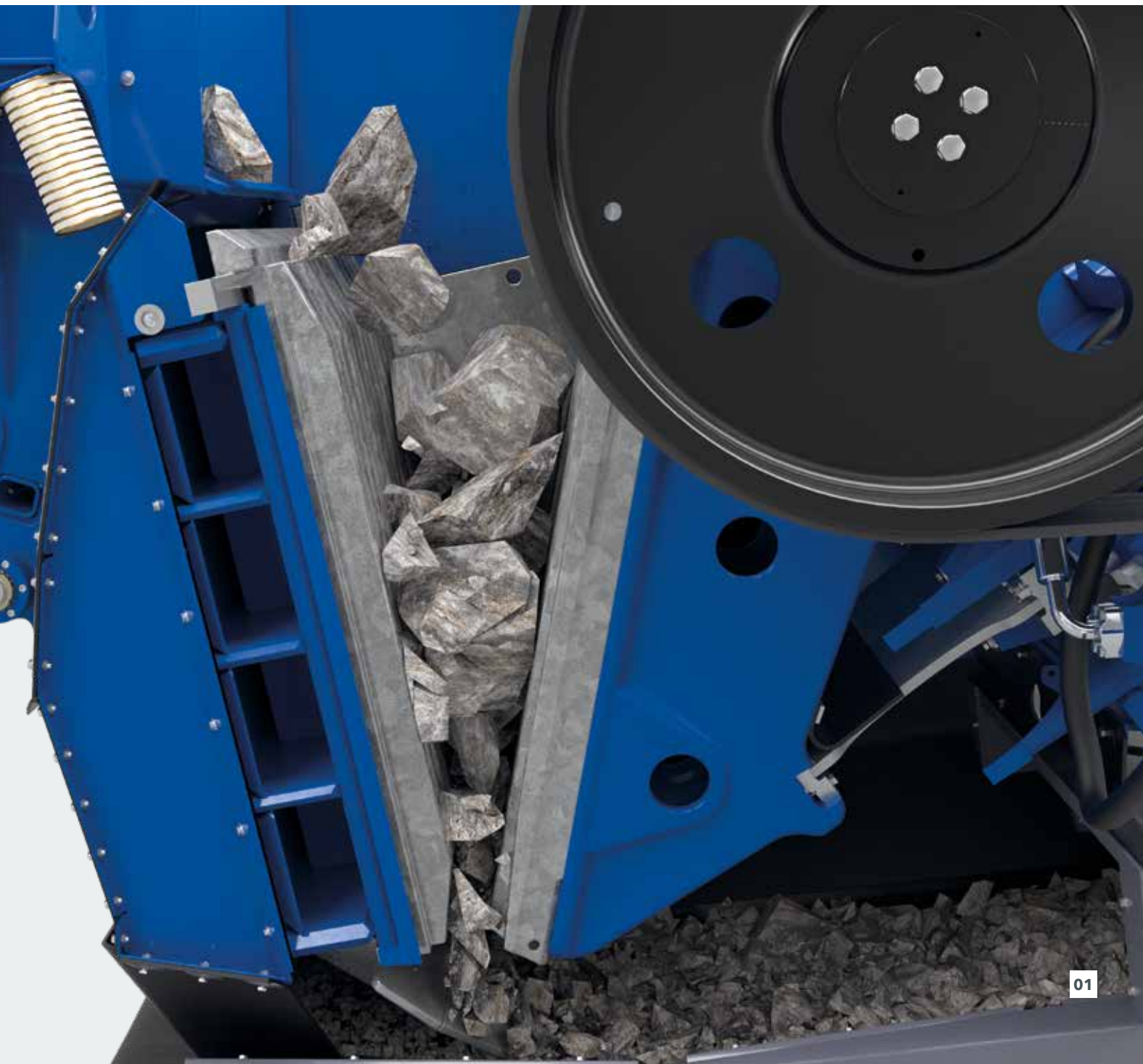
01 Crusher geometry 02 Deflector plate 03 Crusher unblocking system
