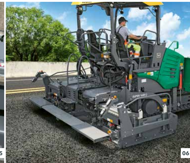
04 All the main paving functions can be controlled via the two handy screed remote control units. 05 Niveltronic Basic System for Automated Grade and Slope Control. 06 Combines with the AB 480 Extending Screed in the TV version.
