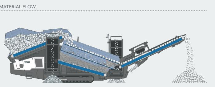
With its proportionally controlled chassis, the coarse screening plant can be moved quickly and precisely, whether from the low-loader to the application site or within the construction site. The side discharge belts can be folded without the need to assemble or disassemble any components, thereby reducing set-up times. More versatility is achieved thanks to a rear hopper wall that
